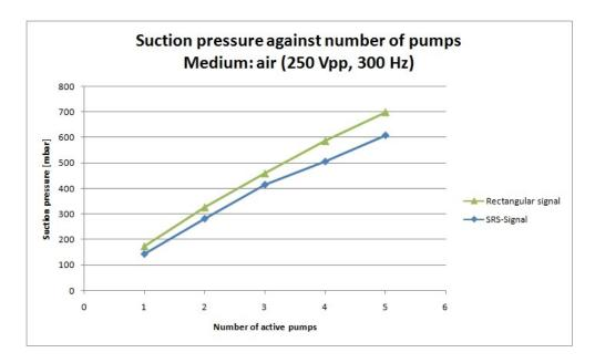
In general it should be noted that the values refer to the performance at optimal driving parameters of the mp6 standard pump. For performance improvement through multiple pumps, please keep in mind the diameter of the tubing suitable for the desired flow, otherwise the advantages gained through multiple pumps are lost to the flow friction of the tubes. Additionally the tubing connectors for stacking pumps in series should be as short as possible to reduce performance loss.
