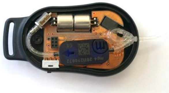
Figure 2: Micropump mp6-AIR integrated in a portable system for NPWT.
